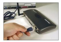
**3.** Plug the large end of the Power cord into an electrical wall outlet, and the smaller end in the Power (marked "12VDC") on the back of the Print Server.
